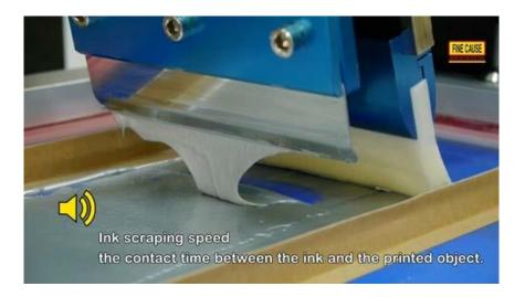
The ink scraping speed depends on the ink. The ink scraping speed should be slower if the ink is thicker or has higher viscosity.
