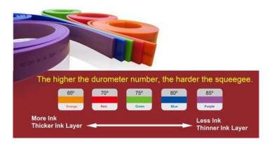
• The harder the <u>squeegee</u>, the smaller the contacted surface with the printed object.The greater pressure applied on the ink, the shorter the contact time with the printed object will be. Therefore, the ink thickness will be thinner, which is suitable for 【finer】 lines.
