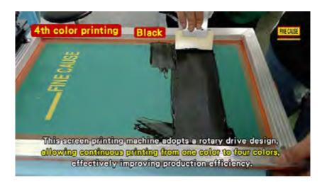
This screen printing machine features a rotary drive design with gas cylinder device, making the printer more convenient and durable to use. It also ensures the stability of print quality.
