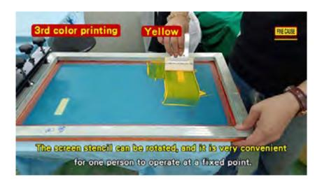
• The screen stencil can be rotated, and it is very convenient for one person to operate at a fixed point.
